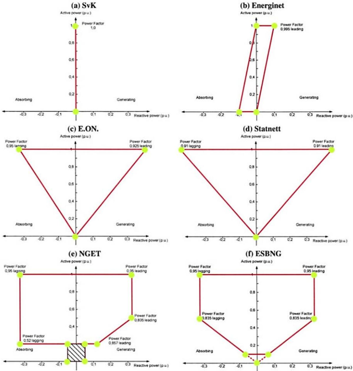
Some grid codes specify the portion of the capability curve that must be dynamic, similar to the AESO standard (Alberta). Some grid codes discuss how this reactive capability may be utilized in operations (voltage/droop control, power factor control, and reactive power control), and the expected response times for each. Some grid codes also discuss the control strategy required during fault conditions, which could play a role in the system design and equipment selection.
