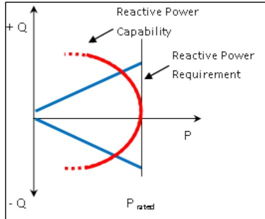
The requirement implied by the blue curve in Figure 8 may not be needed for all transmission-connected PV plants. Considering that most PV plants are relatively small and the output is variable, operation along the red curve or at unity power factor may be just as beneficial to the system as operation along the blue curve. During periods where system conditions warrant, these plants could be instructed to reduce active power output such that a reactive power range can be maintained.
