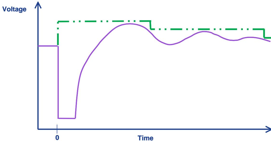
An alternative approach is to specify the cumulative duration at or exceeding the given severity threshold. For example, in the high-voltage case, the duration only needs to include periods when the voltage is elevated.
