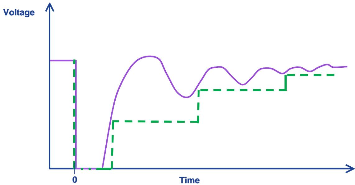
**Figure 13.** Voltage disturbance that crosses the low-voltage criterion envelope.
