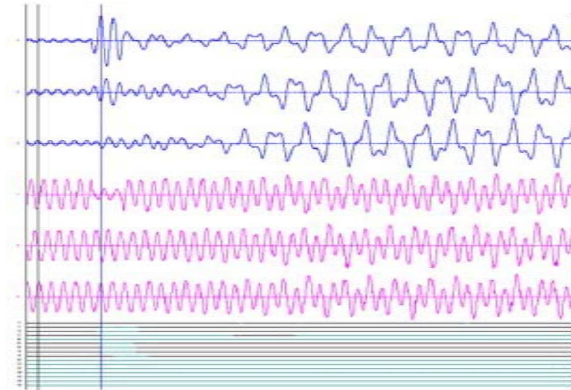
*Note: Triggering event is a single-phase fault. Upper three traces are series capacitor currents and lower three traces are line voltages.*
