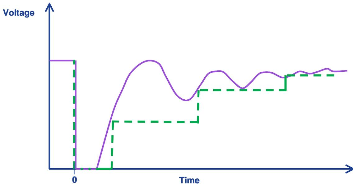
**Figure 14.** Voltage disturbance and high-voltage criteria envelope.
