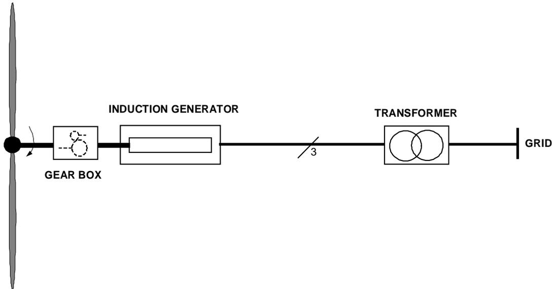
**Figure A3.2.** Type 2 Wind Turbine-Generator: Variable Slip Induction Generator.<sup>21</sup>
