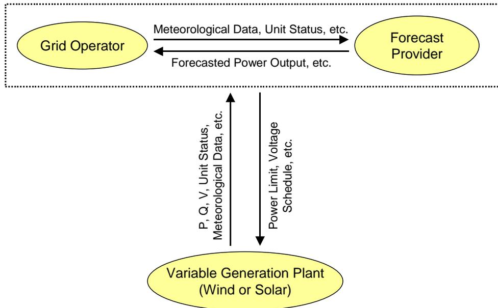
It is understood that a plant operator may be located remotely from the variable generation plant, perhaps in a facility that monitors and operates multiple plants, possibly in multiple operating areas. The point is that the grid operator must have 24/7 access to a person who has direct and immediate control of the variable generation plant.
